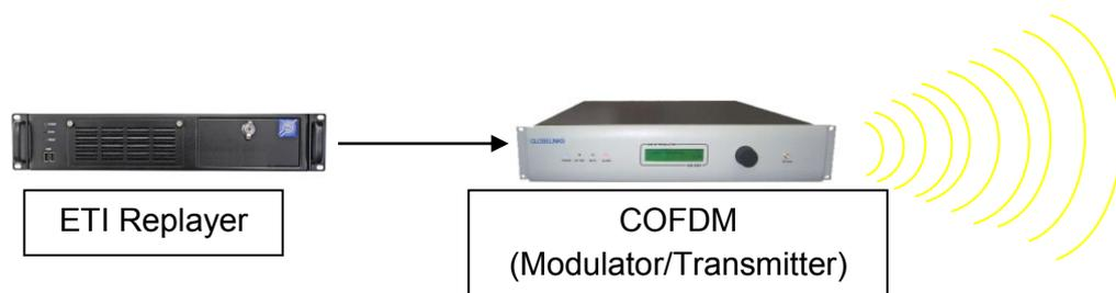
Some modulator/ transmitters that are designed for testing purposes incorporate an internal ETI Player. To play the ETI file you must upload it onto the lab modulator/ transmitter (e.g., via network or USB memory stick) and the lab modulator/transmitter directly plays the ETI file.
