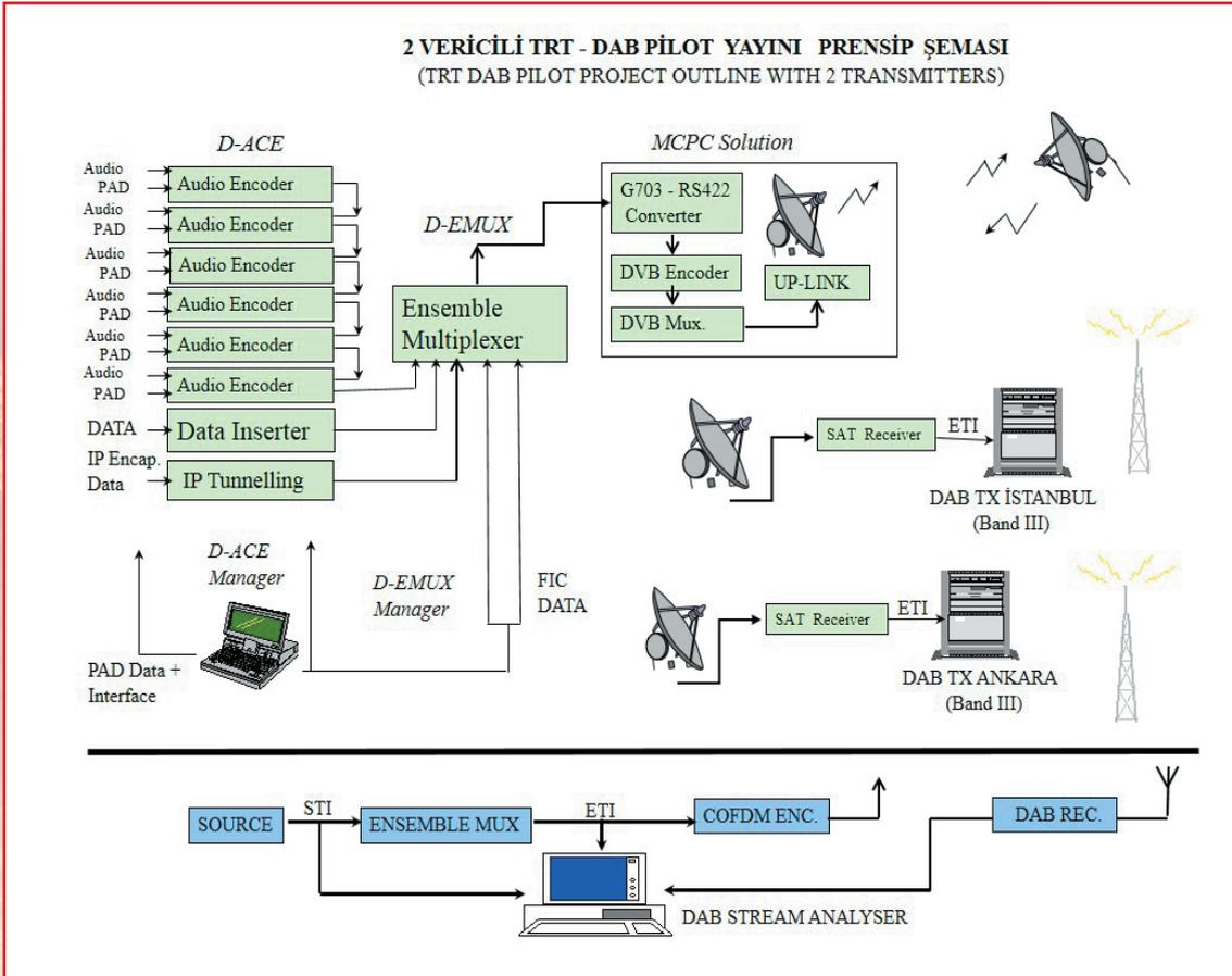
As can be seen in the DAB Pilot Project Principle Schema already existing DVB-S MCPC platform was utilized to convey DAB transmission signal (which includes radio and data services for SFN-Single Frequency Network application) to transmitters via satellite. After confirming the success of SFN application with two transmitters in Ankara, 1kW DAB transmitter was taken to İstanbul in 2007 to promote in fairs and to increase awareness about digital radio broadcasting.
