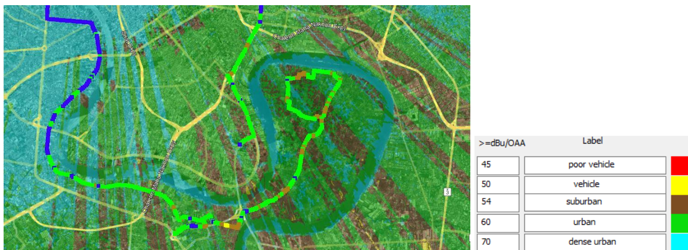
Figure 2: An example coverage prediction showing shadow lines caused by very tall buildings in Bangkok including drive test results track and the field strength palette
