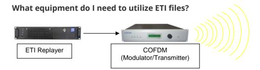
To replay the ETI files to your DAB modulator, you will need an ETI Replayer. Some modulator/ transmitters that are designed for testing purposes incorporate an internal ETI Player. To play the ETI file you must upload it onto the lab modulator/ transmitter (e.g., via network or USB memory stick) and the lab modulator/transmitter directly plays the ETI file.
