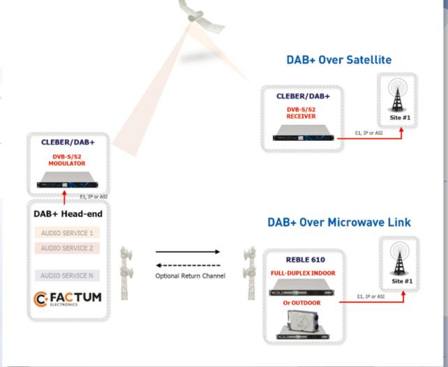
Elber, the Italian distributor of Factum for DAB/DAB+ head-end, is able to provide multiple ETI transport over satellite with its dedicated DVB-S/S2 uplink/downlink system.
