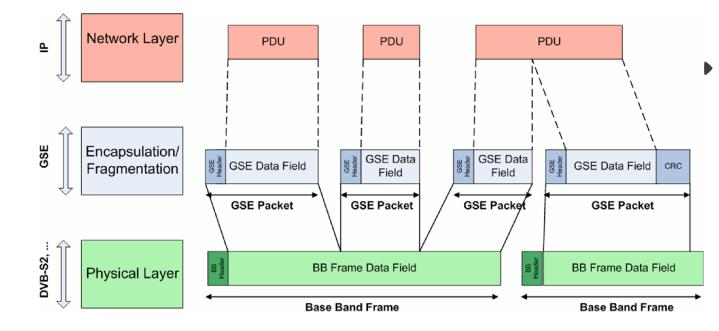
IP Packets are directly copied into the PDU field of the GSE packet. The protocol overhead is minimal.
