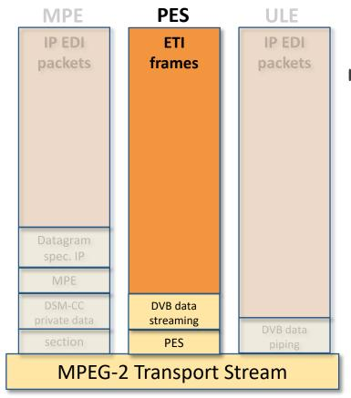
For transmission of ETI Frames (uncompressed or compressed) when no IP EDI is available a Packetized Elementary Stream (PES), similar to audio and video distribution, can be used.
