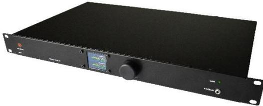
The complete system is realized in the Paneda 1U true all-in-one unit with multiplexer, up to 16x DAB/DAB+ encoders, metadata content server and management built-in. The Paneda 1U offers redundant network interfaces as well as dual power supplies. Audio interface supported is AES/EBU as well as most known IP formats.
