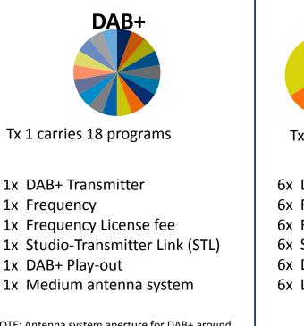
NOTE: Antenna system aperture for DAB+ around 200MHz is approximately 1/2 that of FM and DRM+ around 100MHz for the same gain.
