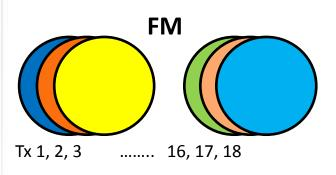
18x FM Transmitter **18x** Frequencies 18x Frequency License fee 18x Studio-Transmitter Link (STL) 18x RDS encoder/ Data 18x Large antenna
