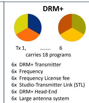
NOTE: DRM+ has a maximum capacity of 186kbps which is equivalent to 62kbps per service using 16QAM and FEC code rate 0.62 15
